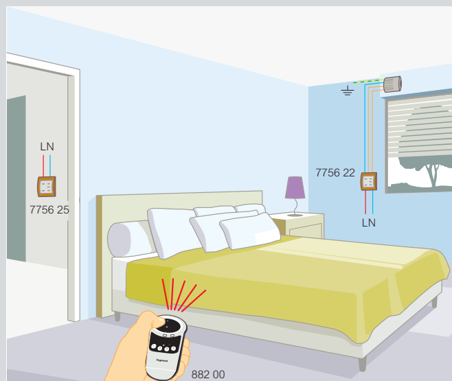
Shutter control in a new building (PLC Solution)
